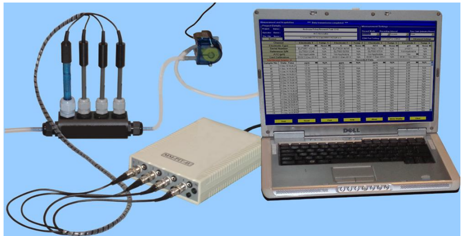
Flow-through Cell with 1xpH, 3x Ion selective Electrodes and 4-channel Monitor
