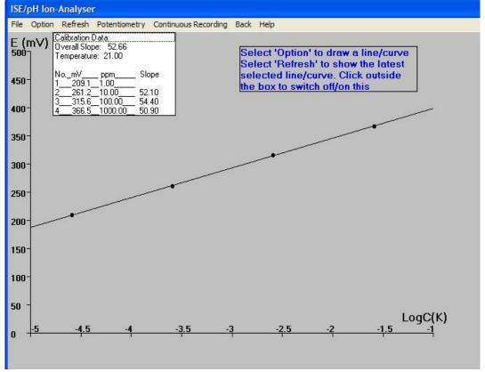
The Potentiometry/Measurement screen is the main working area for ISE measurements. Once a calibration line has been plotted, either from new data or from an old calibration file, the **Option** menu will allow you to change the type of line fitting and change the scales on the graph; but note that only the **Linear Regression** will allow you to measure samples which lie outside the range of the calibration data. Extrapolation is not recommended for the highest precision.
