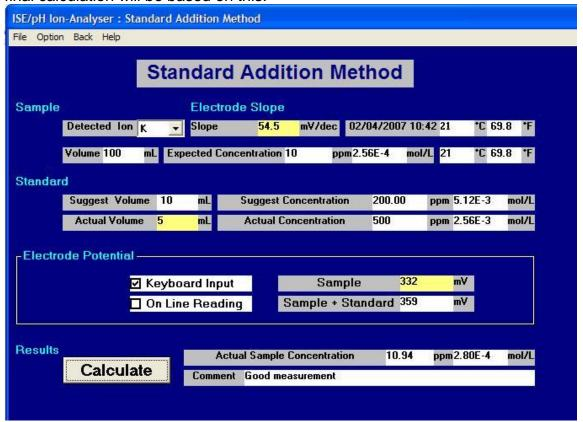
Remember to press Enter after typing in any data to make a permanent record and activate any accompanying calculations.
