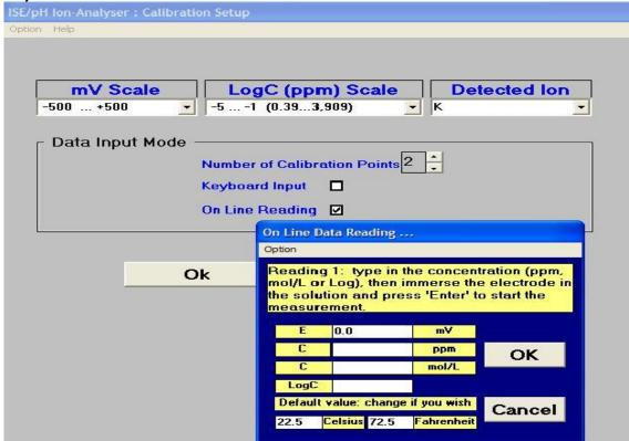
The first screen allows you to enter the parameters for defining the axes of the calibration graph. These are millivolts for the y-axis and the logarithm of the molar concentration for the x-axis (the approximate ppm equivalent is given in brackets as a guide to the concentration range required). If there is any doubt, it is suggested that the widest range is selected initially, since the scales can be quickly changed once the graph is plotted.
