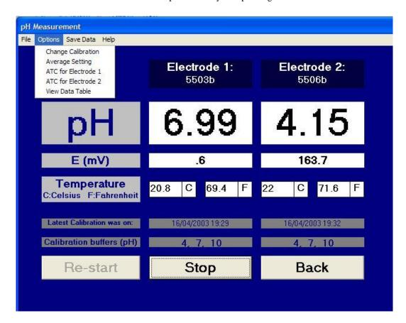
The **Option** menu allows you to load a different calibration from a saved file (**Change Calibration**), change the **Average Setting** (for more precise measurement), switch on or off the Automatic Temperature Compensation in either channel (**ATC**), or **View Data Table**. The File menu can be used for **Print**ing the current data table or **Open**ing and reviewing old data files.
