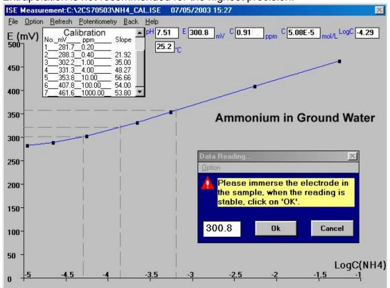
If sample concentrations range over several orders of magnitude, the **Partly Linear** option, which uses the actual slopes between the individual points, will probably give the best results. Note that if you change the type of line-fitting or the scales during a series of sample measurements, the screen will be cleared of any plotted sample lines – but the data will remain in the data table.
